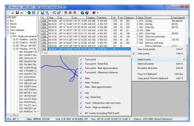
The first filter to apply is to unselect **view track points**. There is also a toolbar item for this. This will hide all the fixes in the analysis frame which have no associated event. Suddenly it becomes much easier to see the stuff you want to analyse, and with the mouse cursor over the analysis frame and with the 'move map to show position' toolbar icon active it is possible to scroll up and down all the events very easily while inspecting them on the map.
