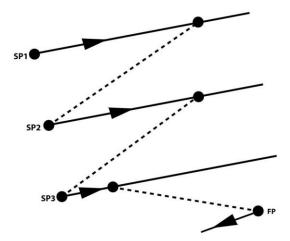
Known track lines will consist of three lines. SP1 is the start of the first known track. Crews should fly this track until finding a photo feature marked as a turnpoint (the letters 'TP' will be in the upper right corner of the photo). From this point they must construct and fly a straight line track to the start point of the second line (SP2),
